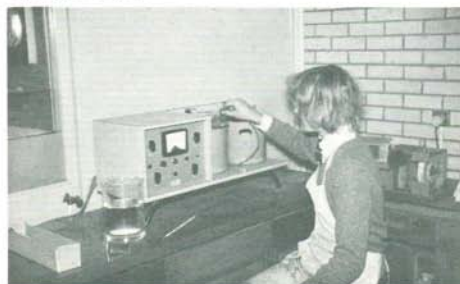
Pupil using electro-plating equipment to nickel plate a copper pendant.
