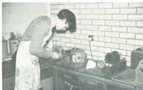
Pupil using a diamond saw on a combination lapidary unit.
